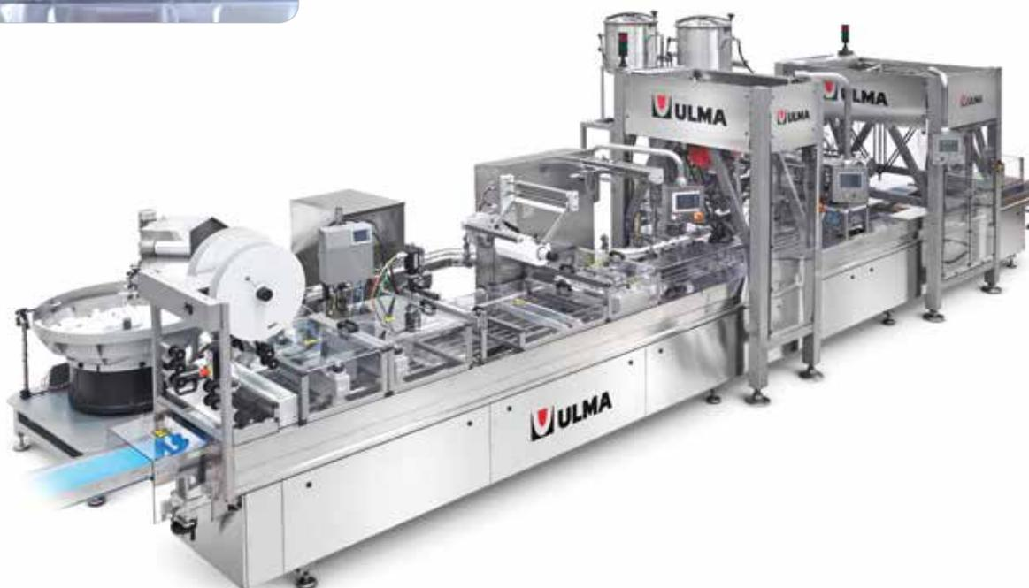
Thermoforming machine with automatic loading and dosing.
